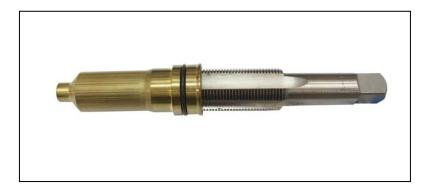
SEPT 2 : Take no.3 & 4 to lock up the old sleeve, and pull out the sleeve.
