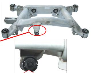
Note: The Sign On The Accessories No.9 Must Be Parallel With The Suspension.
