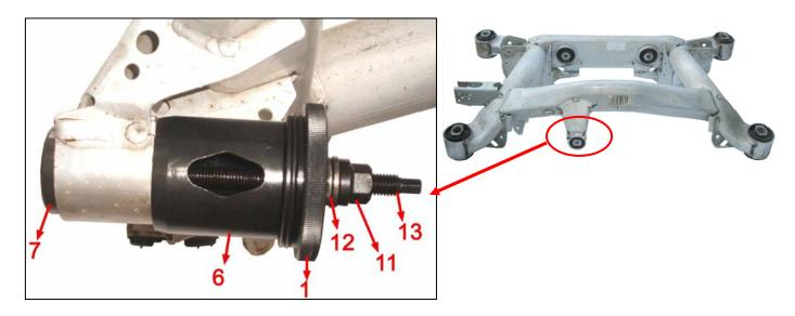
BMW (E38/E39) Front Differential Bush Installation: Step 1: Preparation for Installing The Front Bush
