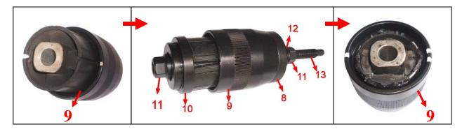
NOTE: The fillister on the bushes and the sign on the accessories No. 9. must be in the same line, and then moved into the accessories No. 9.
