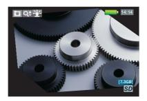
The adjustment of rotation angle has 5°/15°/30° /90°, Press "Enter Button" for choosing these angles and then press "Left/Right Button" after popping up main menu in the screen to choose the related rotation degree in the submenu of the "Rotation", as shown to the right:
